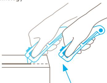
**Fully automatic blade retraction – a very high degree of safety**
